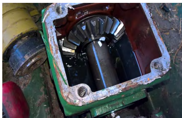
Figure 2 – Worn gearbox (Note mis-alignment of white marks)
